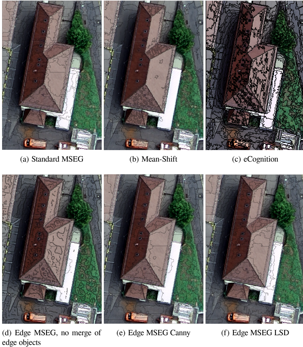
Figure 6.2: Comparing various segmentation algorithms on a DMC aerial multispectral image with 5 cm pixel-size (©Intergraph Corp.). (a) Standard MSEG with scale parameter 100. (b) Mean-Shift segmentation with default parameters. (c) Multiresolution segmentation (eCognition) with default parameters. (d) Edge constrained MSEG, without merging the edge objects in last pass, for demonstration purposes (e) Edge constrained MSEG, employing the Canny edge features. (f) Edge constrained MSEG, employing the LSD edge features.
