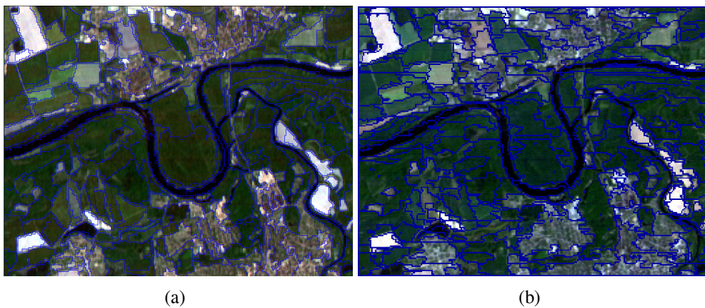
Figure 3.5: Segmentation result by eCognition for scale parameter 20 (left) and texture-based MSEG for scale parameter 2500 and texture parameter 3.0 (right)
