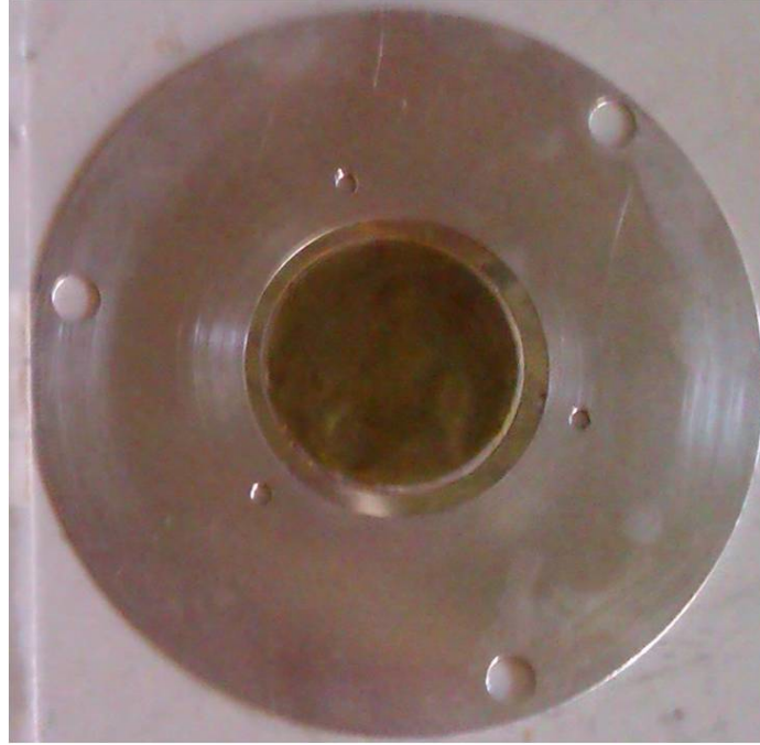
Figure 2.1: The picture of one of the ^{238}\text{U} reference targets (label 210).
