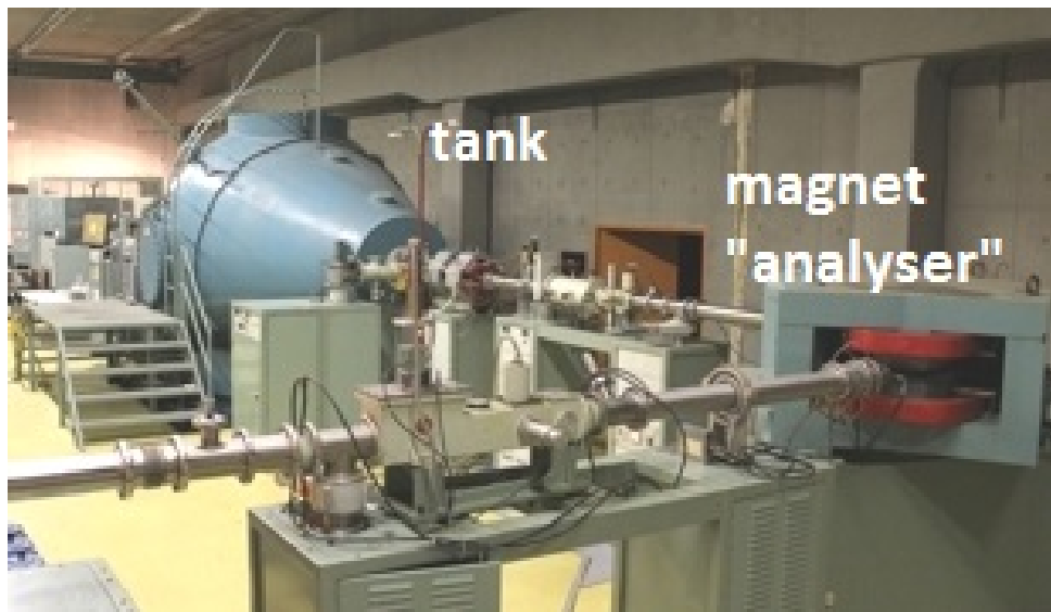
Figure 5.1: Photo of the high energy part of the accelerator system at the Institute of Nuclear and Particle Physics of the NCSR “Demokritos”. Two main parts can be seen: the tank where the 5.5 MV Van de Graaff generator is located and the “analyser” magnet.
