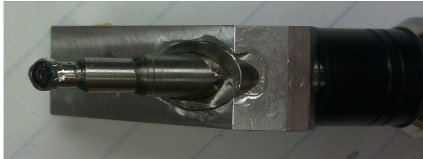
Figure 2.10: A photo of the nozzle that shaped the proton beam, along with the 100 nm \text{Si}_3\text{N}_4 exit window.
