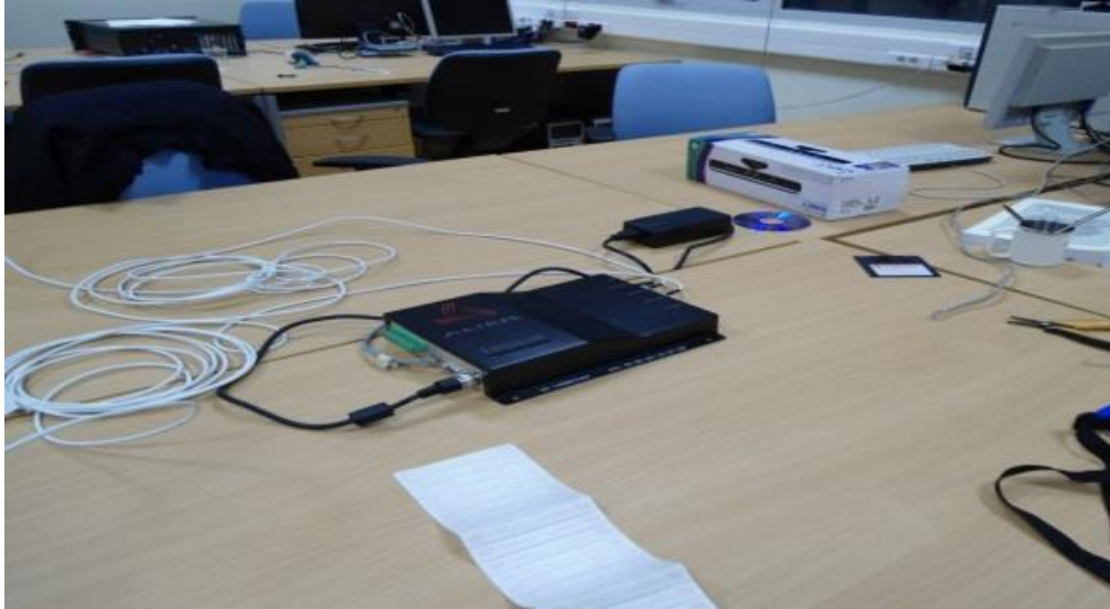
Figure 35: RFID System (the Alien ALR- 8800 RFID Reader).
