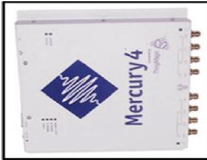
Figure 13: Example of an RFID reader [51].
