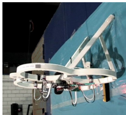
FIGURE 1.2: A quadrotor applying force to a wall [7]
