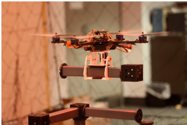
FIGURE 1.4: A Quadrotor equipped with a gripper from UPEN Grasp Lab [12]
