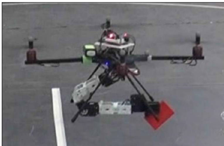
FIGURE 1.11: A quadrotor with 2 DoF manipulator in [26]
