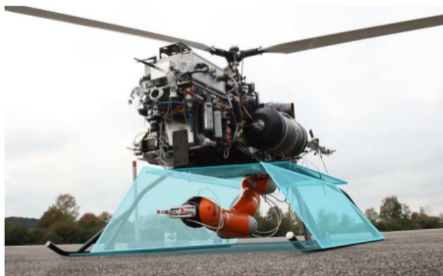
FIGURE 1.8: A helicopter equipped with a 7 DOF robotic arm in [19]
