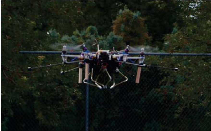
FIGURE 1.9: A novel dextrous hexrotor manipulator in [21]
