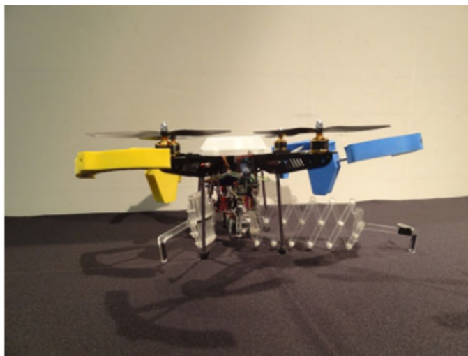
FIGURE 1.12: A quadrotor with three 2-DoF robotic arms in [27]
