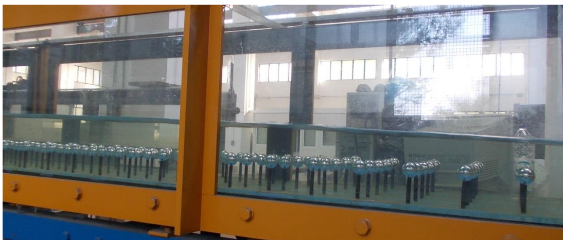
Picture 3: Experiment Type III, density 100 stems/m 2 , 60 l/s
