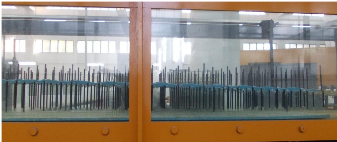
Picture 2: Experiment Type II, density 200 stems/m 2 (staggered), 40 l/s
