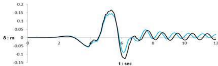
e) Deck Displacement - time
