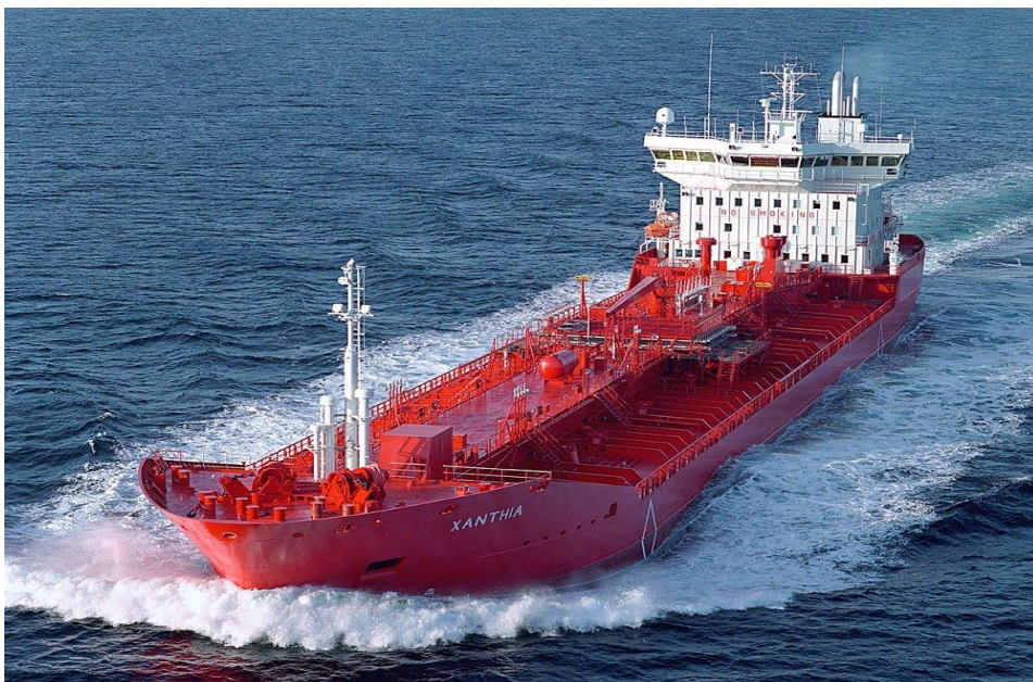
Figure 2.2. Typical chemical tanker
