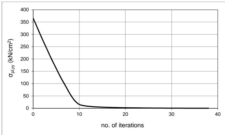
Figure 6.40 Evolution of the yy component of the plastic stress vector \sigma_{pl}^{cs} at GP2 (time 3T/4 , (P_1^*/P_2^*)=(1/1) )
