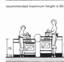
19 Plinth depth varies height of work surface
