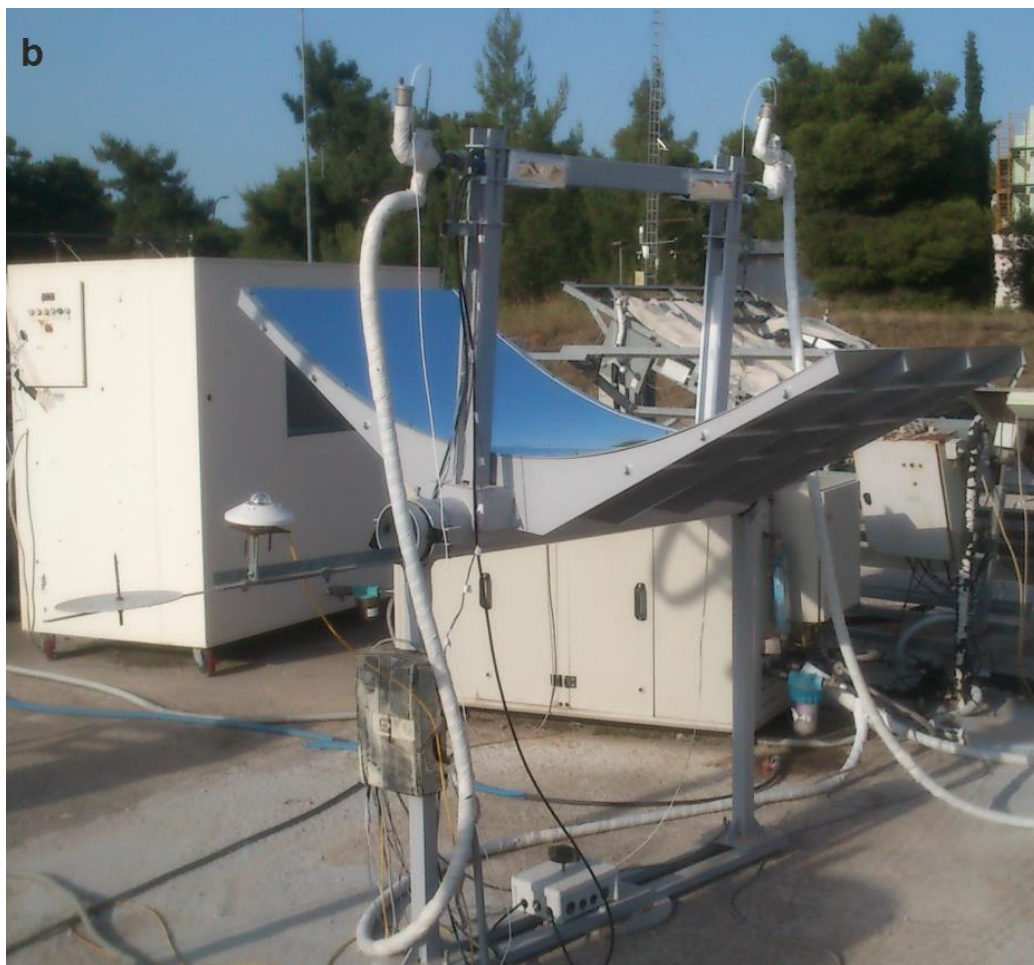
Fig. 5.5 Metallic structure of the CPVT system: (a) CAD drawing and (b) photograph showing the frame constructed along with the main hydraulic and electrical connections.
