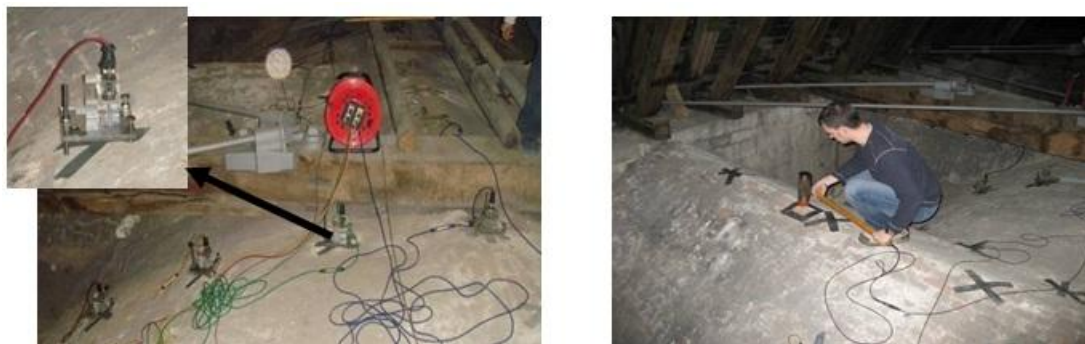
Figure 3.16 The measurement axis of the accelerometer (Q-Flex QA 750 model force balance accelerometers) is aligned vertically by adjustable screws (Pavic et al. 2002).
