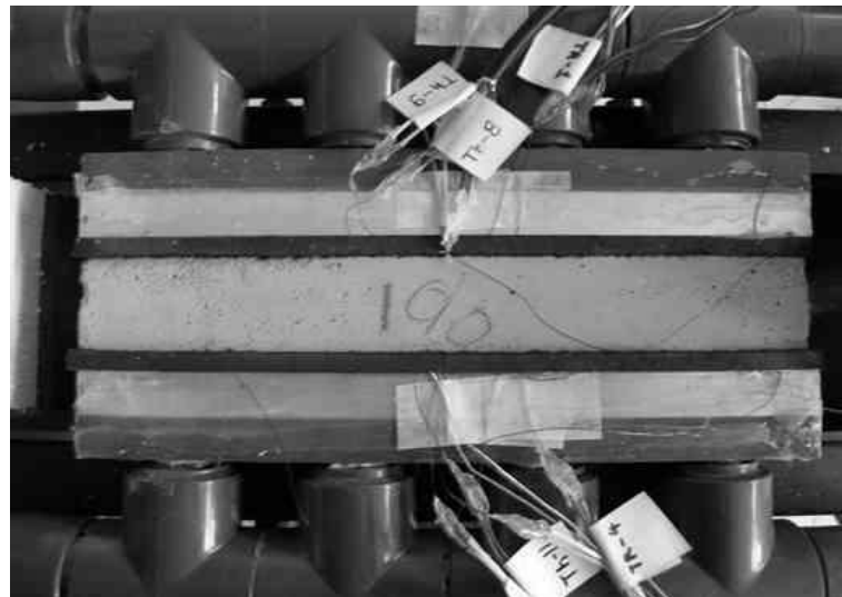
Figure 5.8: The configuration of the concrete specimen inside the sample holder of the DHMA. The insulation layers are placed between the plates and the specimen.
