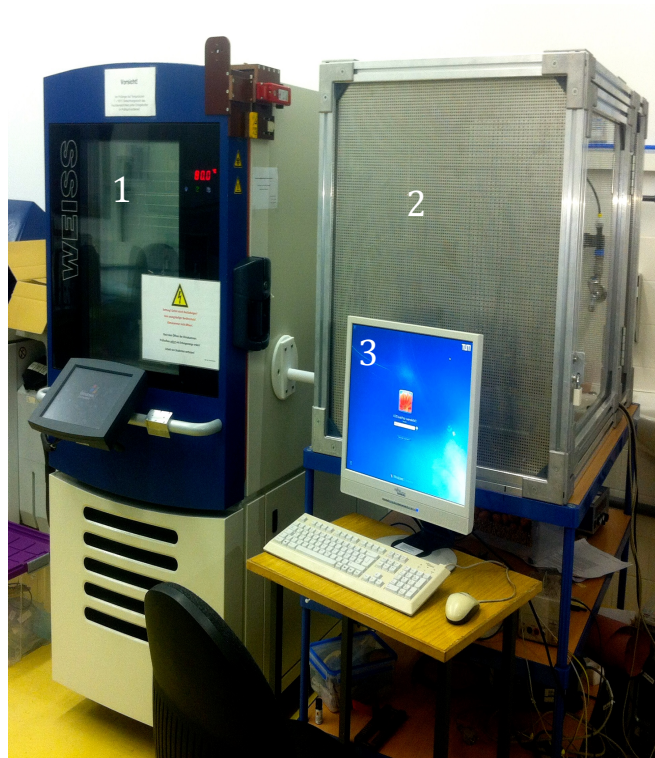
Fig. 5.2: Test arrangement for Conduction Current Measurements on Al 2 O 3 -filled epoxy plaque specimen, in the laboratory of High Voltage Engineering and Switchgear Technology of TUM, showing: (1)The climate chamber, (2) The grounded cage, (3)The computer
