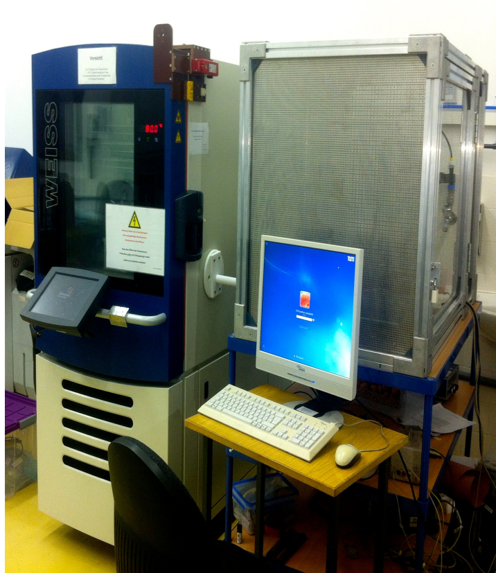
Σχήμα 5: Test arrangement for Conduction Current Measurements on Al_2O_3 -filled epoxy plaque specimen, in the laboratory of High Voltage Engineering and Switchgear Technology of TUM, showing: (1)The climate chamber, (2) The grounded cage, (3)The computer
