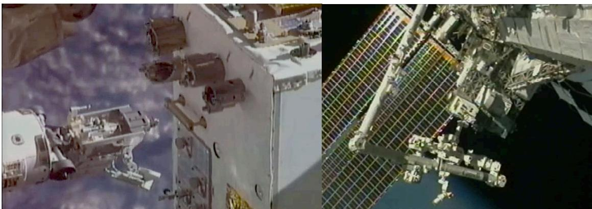
**Figure 1-8.** Dextre robot moves the RRM Multifunction Tool towards the RRM module (left) and the Dextre robot performing a new set of satellite-servicing tasks on the RRM module, during the second part of the Gas Fittings Removal task (right), (source: NASA).
