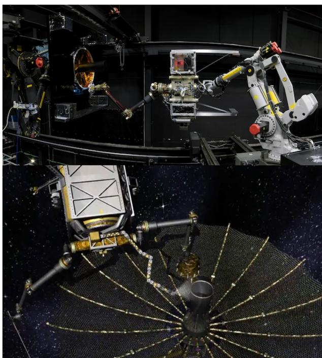
**Figure 1-13.** The FREND under full-scale rendezvous and autonomous robotics grapple testing (top), (source: Naval Research Laboratory) and an artist's representation of the PHOENIX OOS program (bottom), (source: DARPA).
