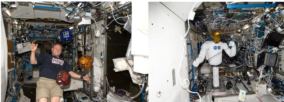
**Figure 1-9.** Robotic systems tested inside the ISS. On the left, Expedition 18 crewmember Michael Fincke as he works with SPHERES in the US Laboratory of the ISS. On the right, Robonaut 2 humanoid robot holds an instrument to measure air velocity during another system check out in the Destiny laboratory of the ISS. (source: NASA).
