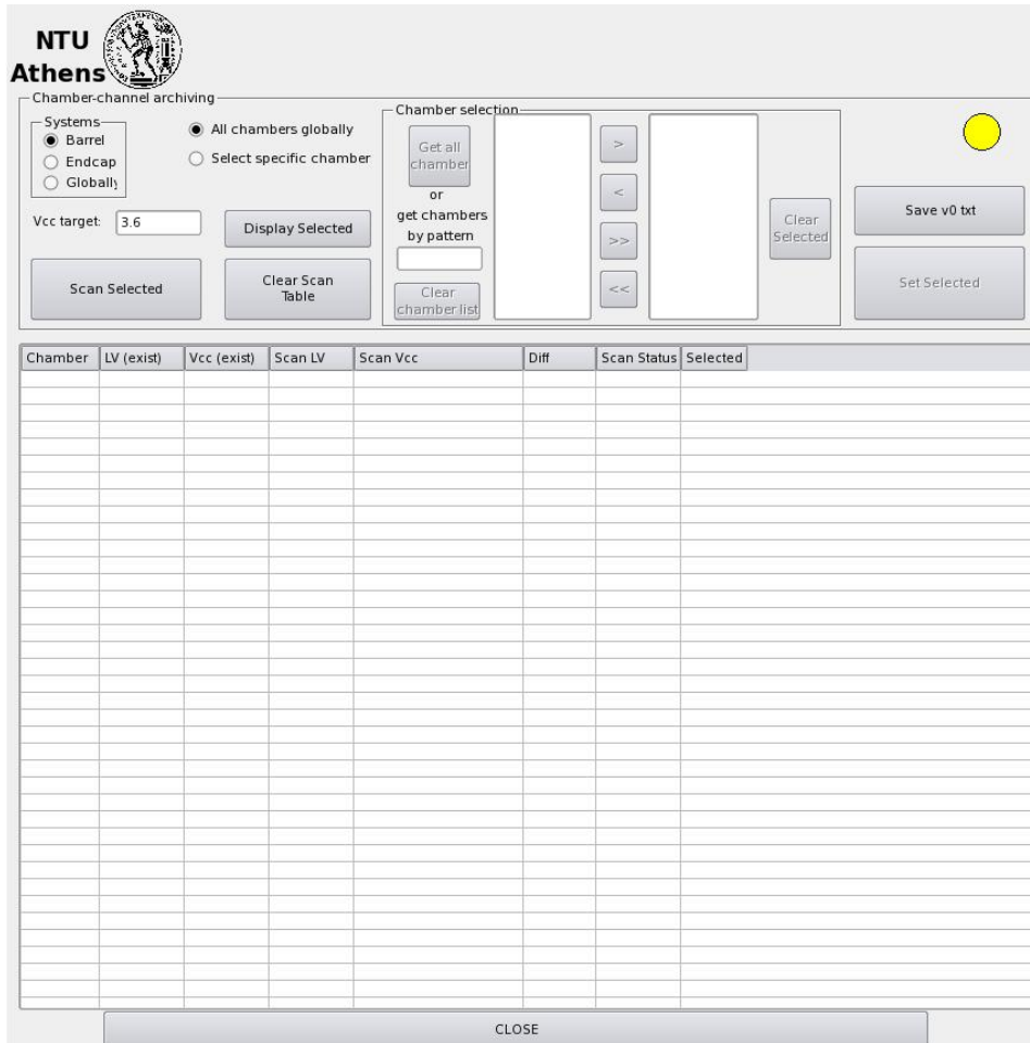
Figure 3.9: The LV scan panel is the tool to be used in order to find the optimum value for the LV of the electronics of the chambers.
