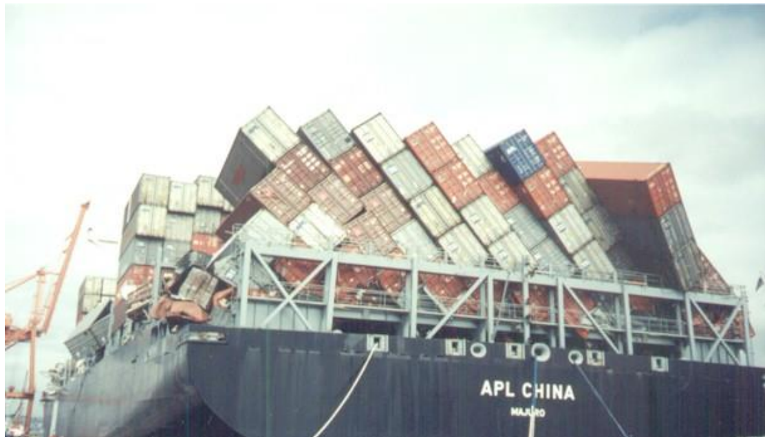
Figure 6: APL China after extreme parametric rolling in rough seas [34]
