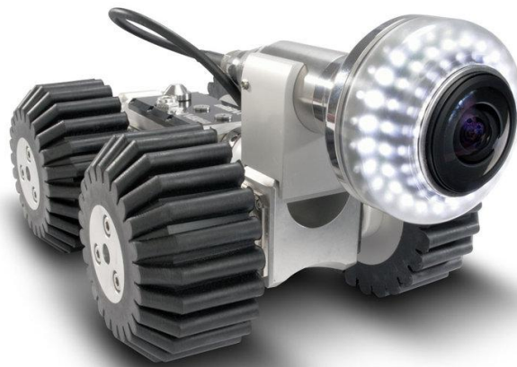
Figure 2.3: CCTV robot, “Digi Sewer” by IPEC (Source: www.ipec.at )
