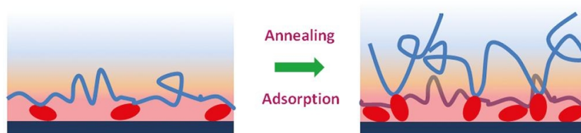
Fig. 1.5. Schematic for the detected two different kinetic regimes during the adsorption of polystyrene on aluminum surface by thermal annealing at temperatures above T_g , taken from [Rotella11].
