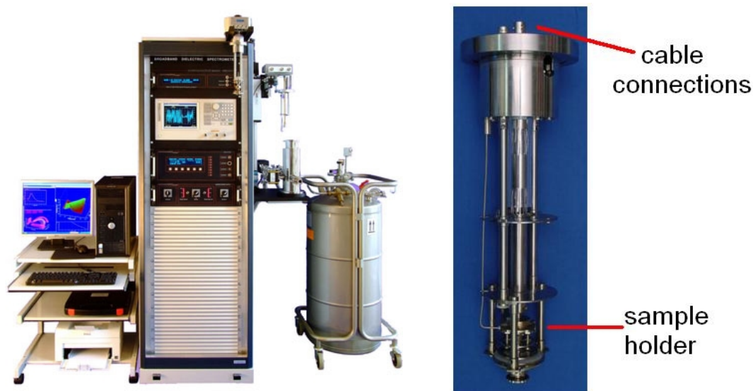
Fig. 3.4. Novocontrol TSDC apparatus in combination with quatro cryosystem and liquid nitrogen cooling system (left) and Novocontrol TSDC sample holder (right).
