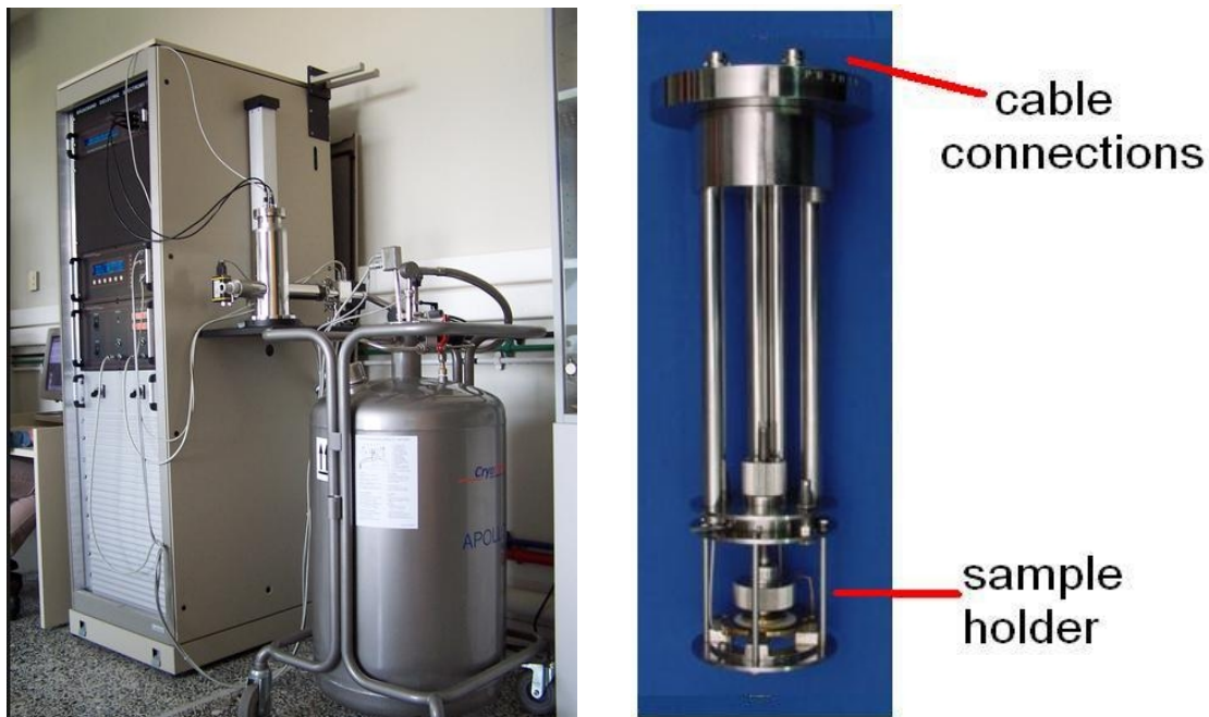
Fig. 3.6. Novocontrol DRS apparatus in combination with quatro cryosystem and liquid nitrogen cooling system (left) and Novocontrol DRS sample holder (right).
