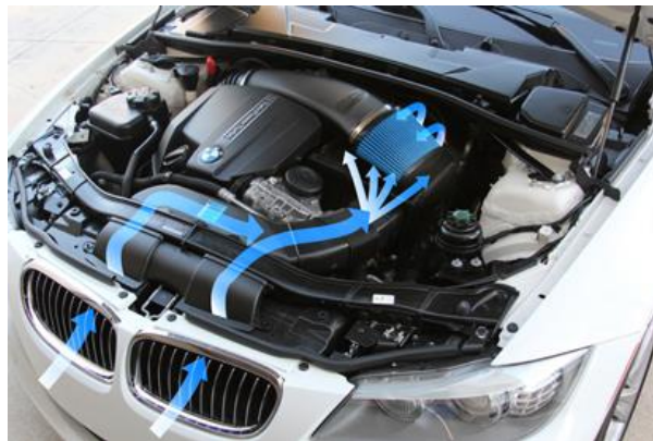
Figure 1.2 The positioning of the air intake system for a conventional car
