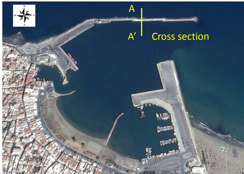
Figure 9: Selected cross section of the breakwater for estimation of wave overtopping.
