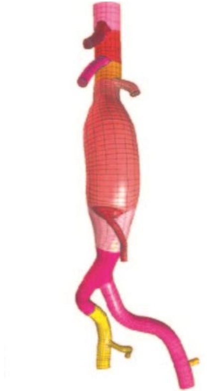
(c) Isogeometric Analysis Toward Integration of CAD and FEA with color-coded patches. The computational mesh consists of 44,892 quadratic NURBS elements.
