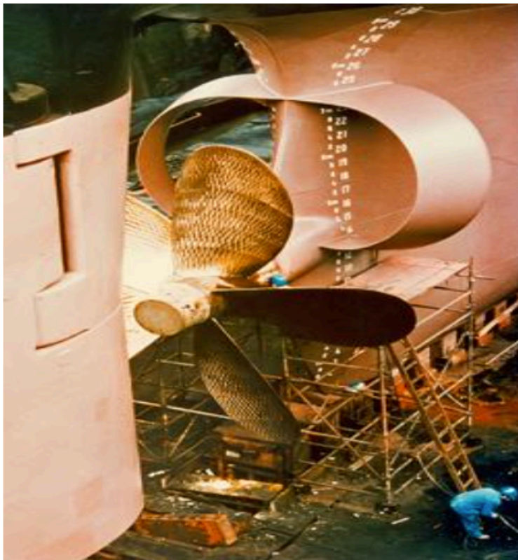
Picture 2: A Wake Equalizing Duct
