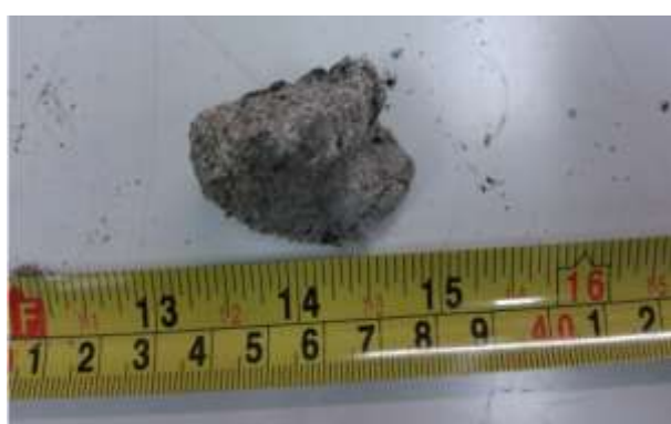
Figure 4.10. Photograph of an indicative agglomerate of magnesite joined particles with cardoon ash.
