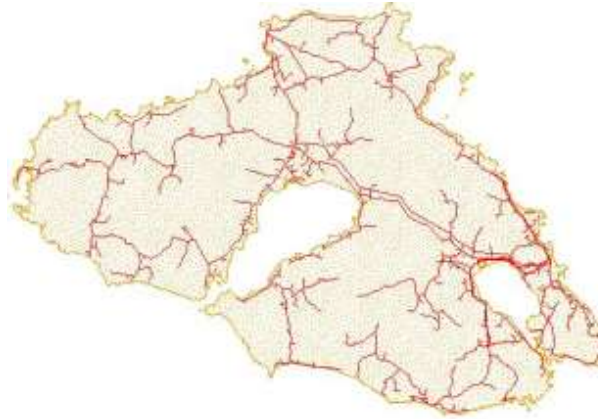
Figure 7.1. The map of Lesvos and the power distribution network of the island [102]
