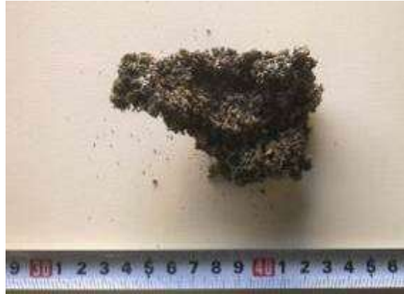
Figure 4.5. Photograph of an indicative agglomerate of olivine joined particles with cardoon ash.
