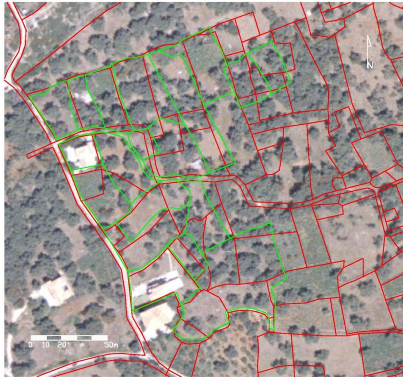
Figure 7-2: Cadastral survey produced by the contractor (in red); cadastral survey produced by NCMA S.A. (in green).
