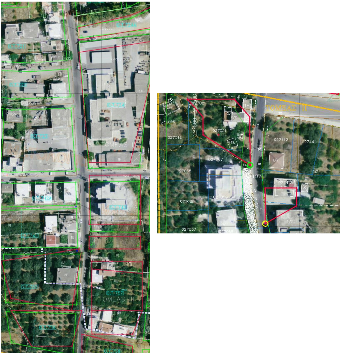
Figure 7-19: The measured land parcels in red. The most precisely measured point in green (0.45 meters) and the most remote in red (13.75 meters)
