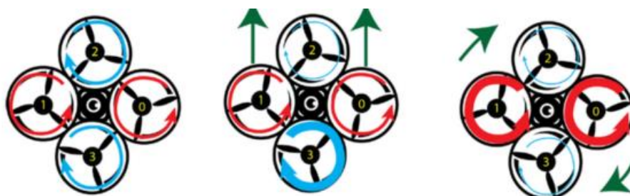
Σχήμα 4.14: hover, forward pitch, right yaw (Leasure et al., 2015)
