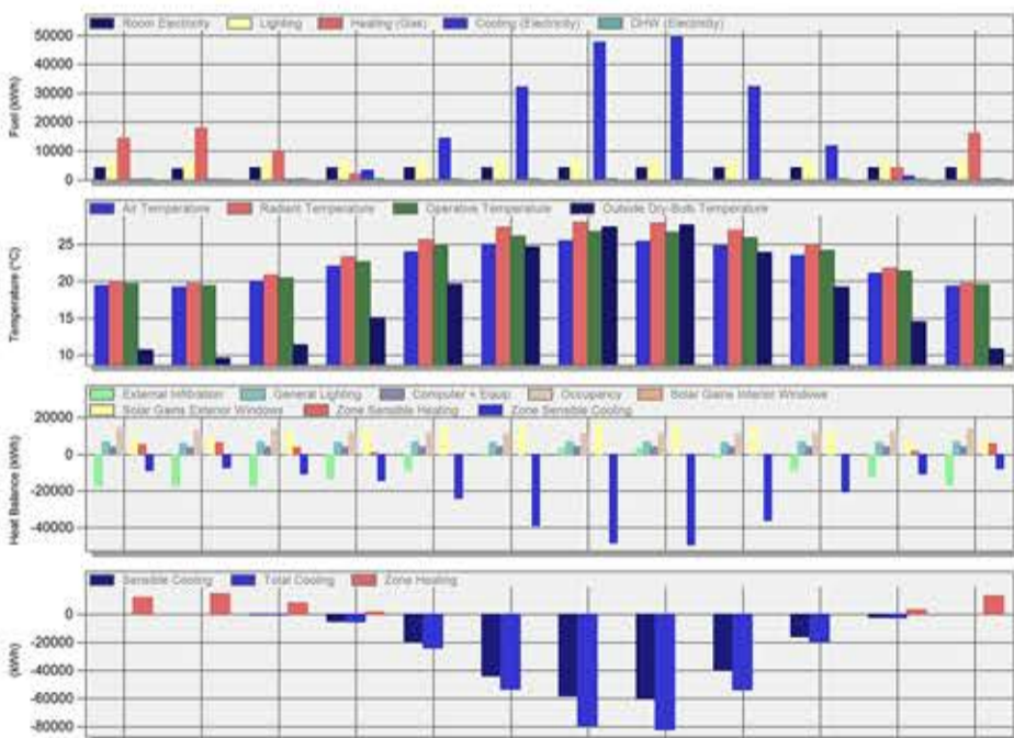
Monthly Temperatures, Heat Gains and Energy Consumption - Athens, Museum Building 1 Jan-31 Dec
