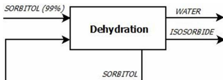
Figure 18: Process of the conversion of Sorbitol to Isosorbide
