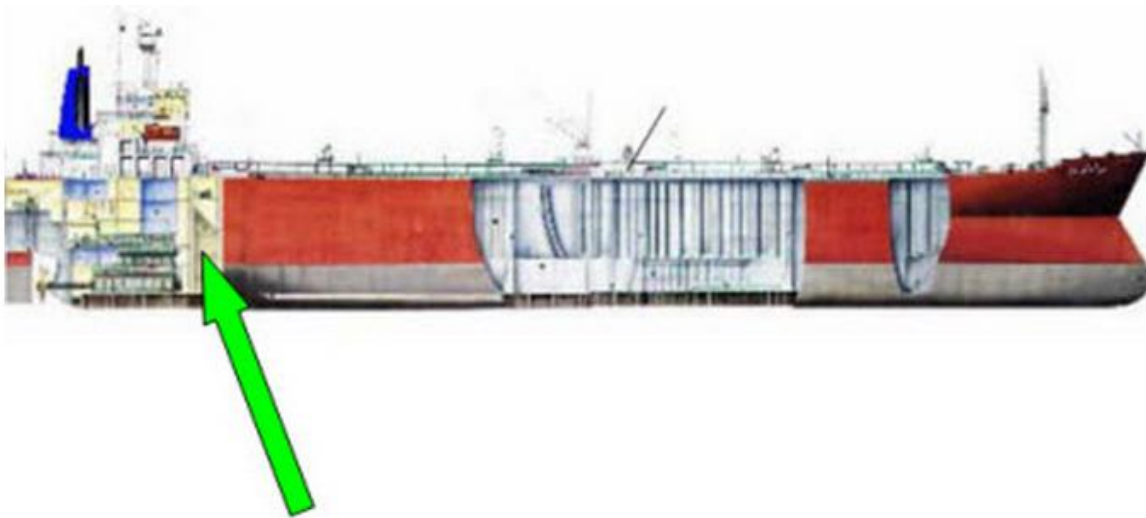
Figure 3.16 – Cargo Pump Room
