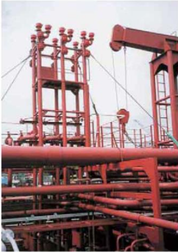
Figure 7.22 – Controlled tank venting system
