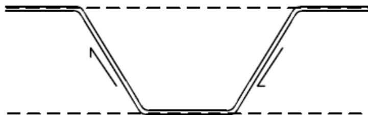
Figure 6.24 – Inner bottom support non-stool bulkheads
