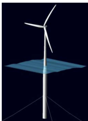
Figure 3.26: Illustration of the OC3 phase IV spar-buoy OWT [figure taken from [94]]
