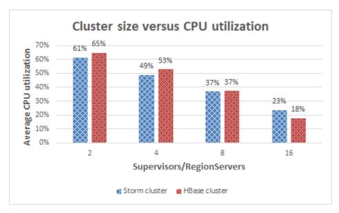
Figure 5.13: Average CPU utilization during scalability experiments
