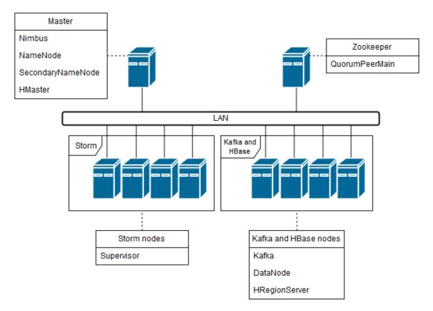
Figure 5.1: Cluster deployment diagram
