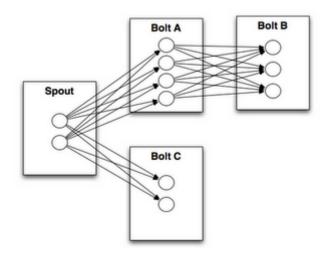
Figure 2.6: Task-level execution of a topology
