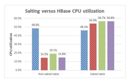
Figure 5.9: Salting effect on HBase cluster CPU utilization
