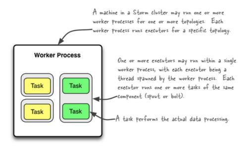
Figure 2.5: The relationships between worker processes, executors and tasks
