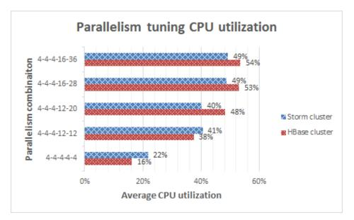
Figure 5.6: Average CPU utilization for the Storm and HBase clusters during parallelism tuning experiments
