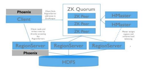
Figure 2.11: Phoenix and HBase architecture
