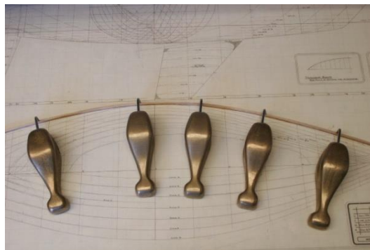
Figure 1.7. Original splines and weights (called Ducks). ( http://www.boatdesign.net )
