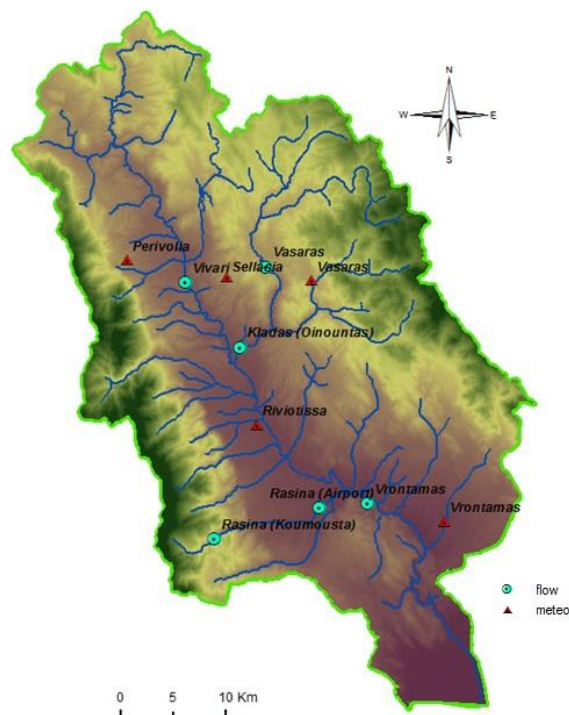
Figure 3: Meteorological (red triangles) and Flow (blue circles) gauging stations in Evrotas river basin
