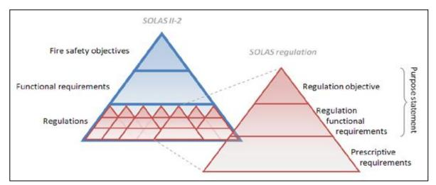
Figure 3.3. Each regulation in SOLAS II-2 consists of a purpose statement and prescriptive requirements. The purpose statements comprise regulation functional requirements and an individual regulation objective which sets out the objective of the functional requirements (Evegren 2015)
