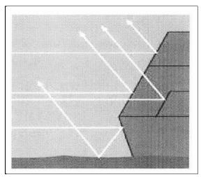
Figure 3.14. The extremely flat, outward-stopping CFRP hull of Visby results in controlled and favorable reflection of radar waves (www.kockums.se).
