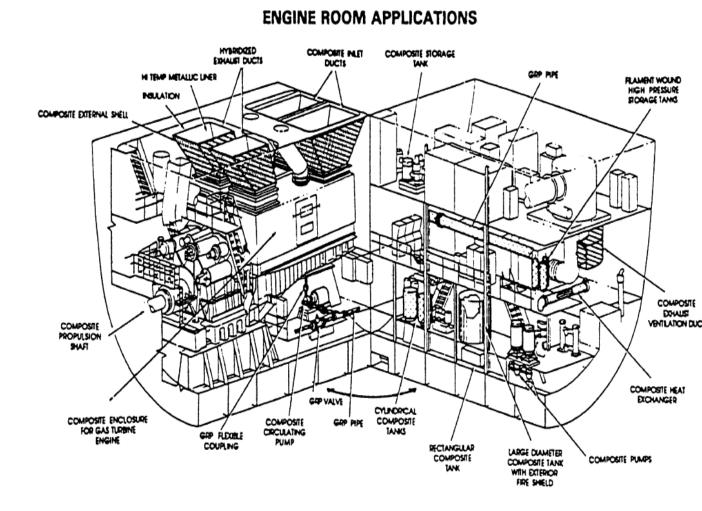
Figure 2.1. Applications for composites in ship machinery compartments (Mouritz 2001)
