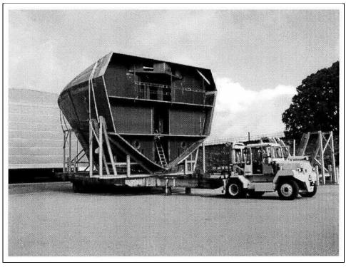
Figure 3.18. Bow section of the Visby-class corvette under transportation to the outfitting workshop (www.canit.se)
