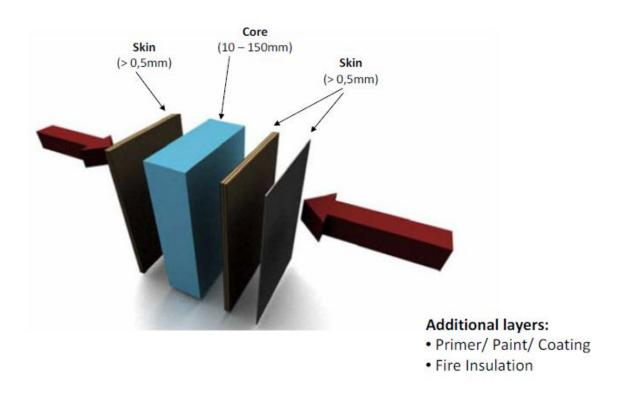
Figure 2.5. Composite layers (Wenstrom 2008)
