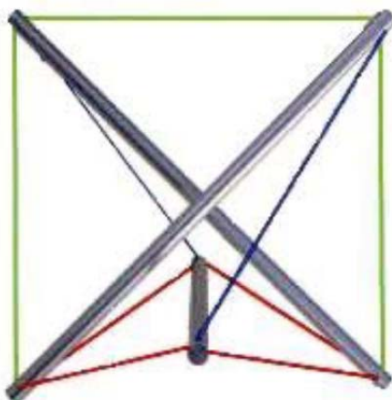
Σχ.4.54 Η βασική tensegrity μονάδα (tensegrity prism)
