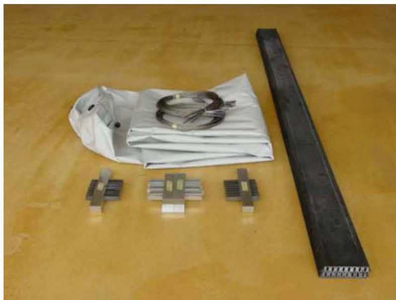
Fig 4.50 Dismantled Tensairity beam of the 8 m span bridge. The compression element on the right is the only bending stiff element, which can be divided in short pieces if compact transport in a box is needed.
