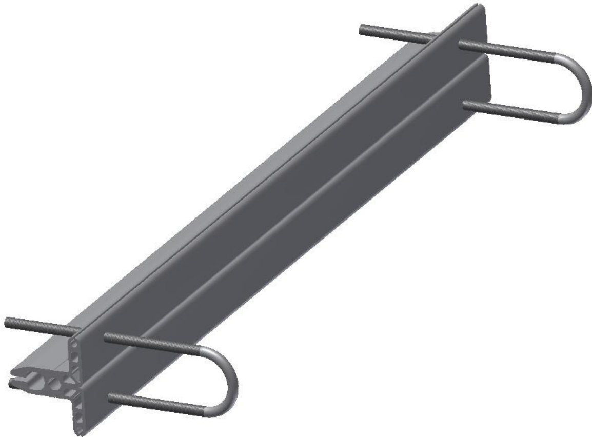
Bracing with U-bolt pipe hanger
