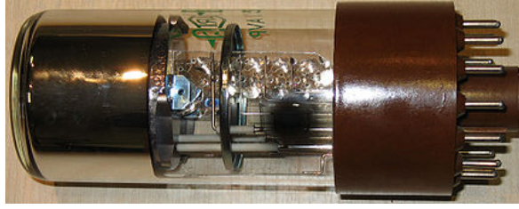
Figure 3.6: A photomultiplier tube and its dynode chain [Wik04].
