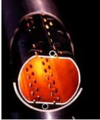
Figure 1.8: The LHC beamscreen: slits in the screens allow residual gas molecules to be pumped out and frozen to the walls of the ultra-cold beam pipe.(image courtesy:CERN)
