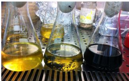
Figure 5. LB medium without CNTs (left), with pristine CNTs (middle) and with commercial CNTs (right).
