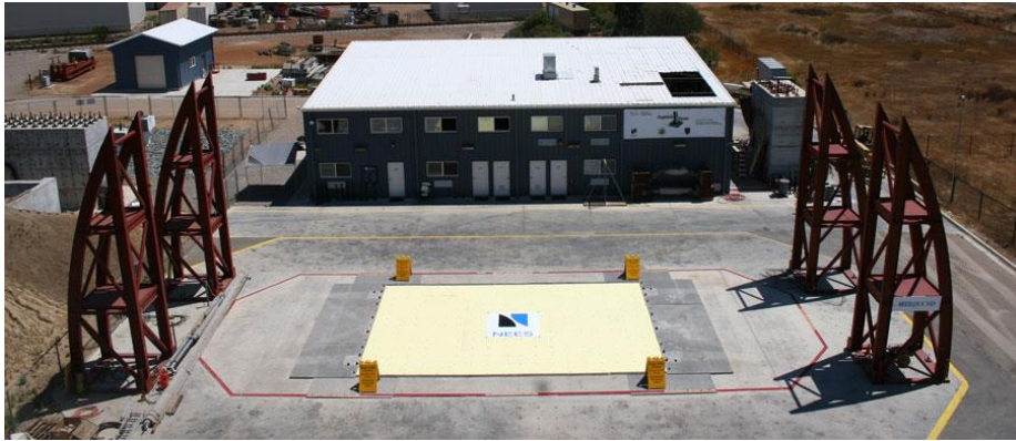
Figure 2.76 The LHP Outdoor Shake Table at the University of California, San Diego. (Source: http://nees.ucsd.edu/facilities/shake-table.shtml )
