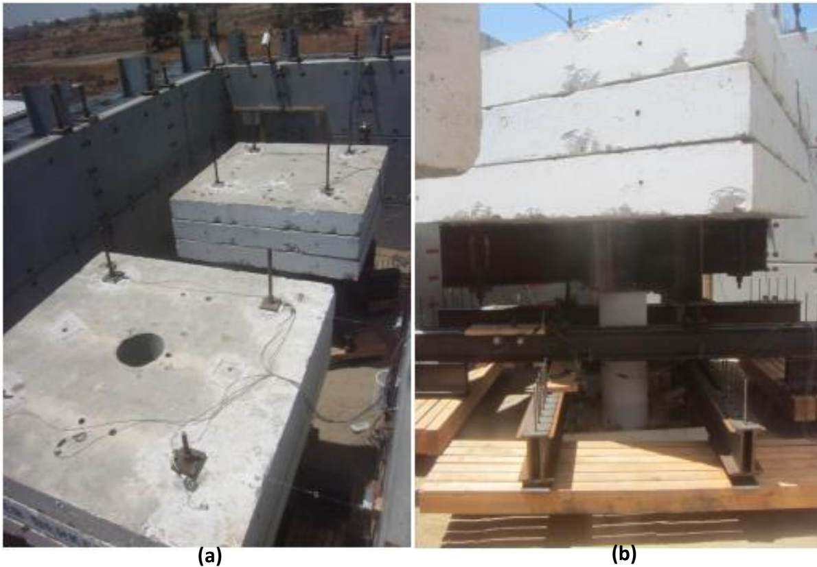
Figure 2.74 (a) Full view of the tested setup (b) system of tapered timber beams fixed to the steel beams allow the “restraining system” to touch the sand surface when the footing rotations exceed values of 10 to 15%. (Fox et al. [2014])
