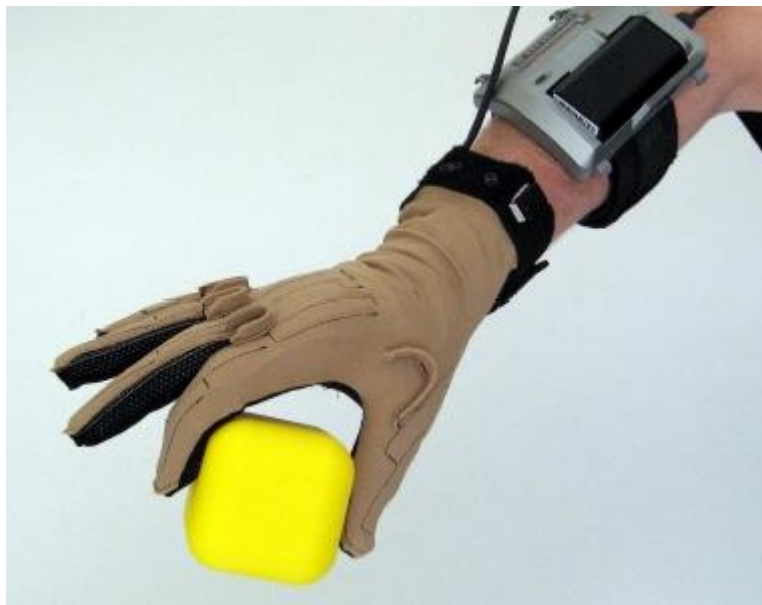
3-1 The CyberGlove II, CyberGlove Systems
