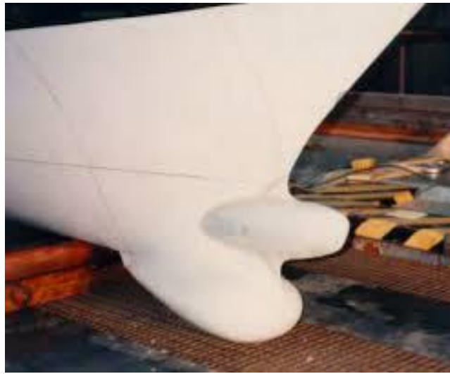
Figure [41]: Model fitted with both a sonar dome and a bulbous bow.
