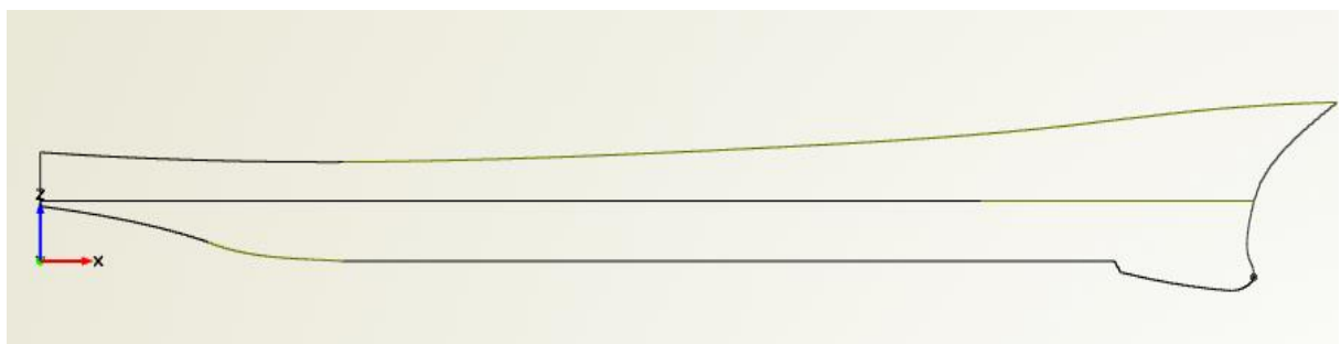
Figure [21]: Centerline, waterline and deck curves.
