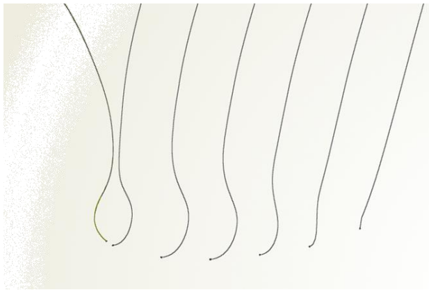
Figure [76]: Bow's profile curve and sections describing sonar dome's geometry.
