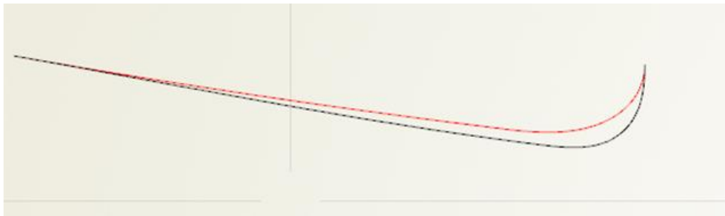
Figure [23]: Changes of two selected design variables and the resulting lower profile curve (initial profile curve with red lines, xz plane).
