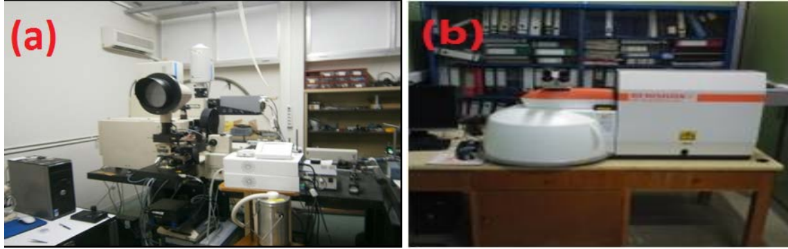
Figure 6 chapter 2. Raman spectroscopy equipment used, (a) at NTUA and (b) at Demokritos.
