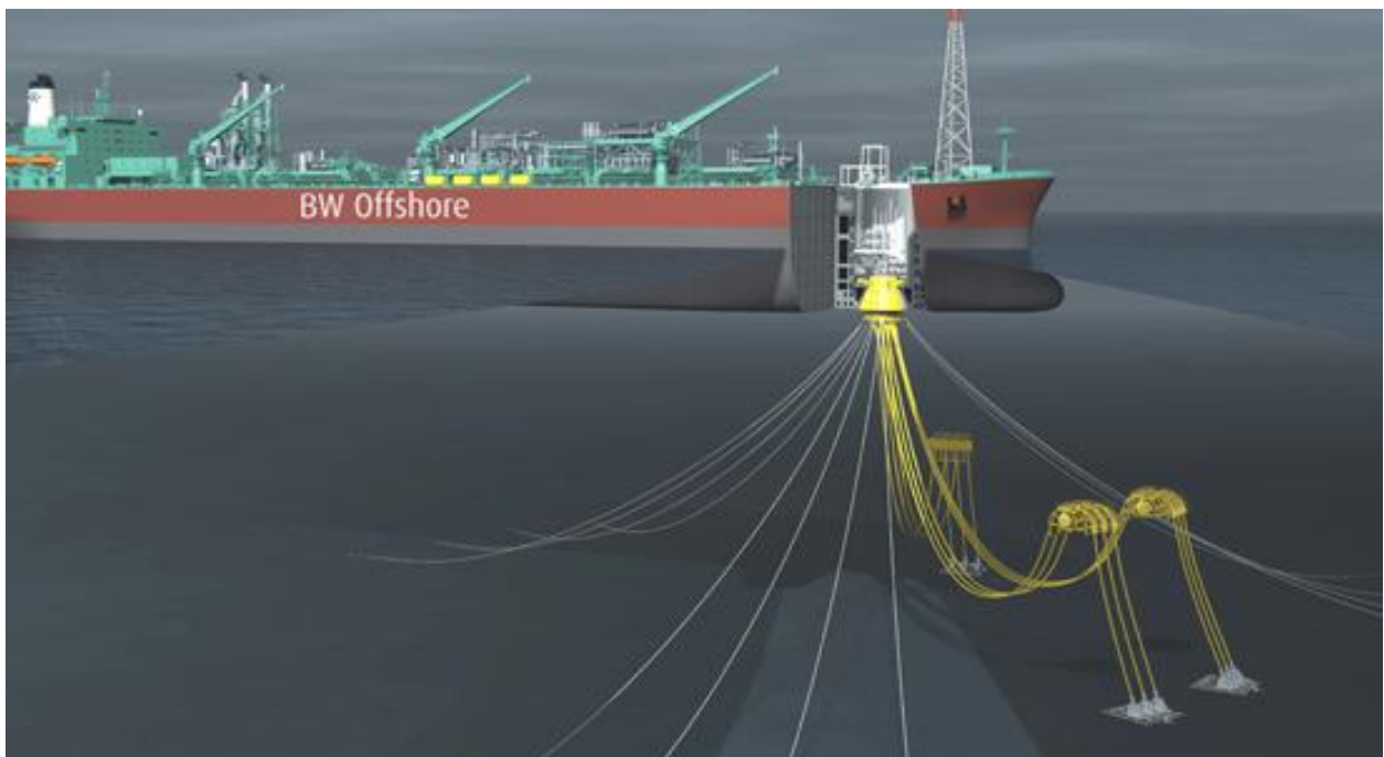
Εικόνα 1-12: FPSO with Internal disconnectable Turret mooring system ( http://www.nov.com/fps_landing/products/submerged-turret-production.html )
