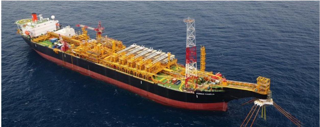
Εικόνα 1-11: FPSO with External Turret mooring system ( http://www.londonmarine.co.uk/ )
