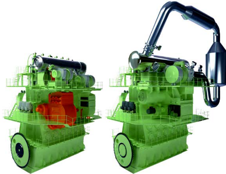
Figure 19: Two-way approach for Tier III engine - EGR and SCR solutions (MAN Diesel & Turbo, 2015)
