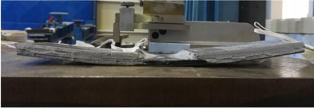
Figure 2.11: Permanent deflection of the specimen
