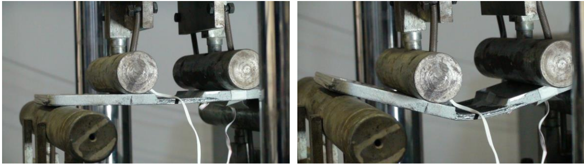
Figure 2.38: Specimen before and during testing (CFRP on the compression side)
