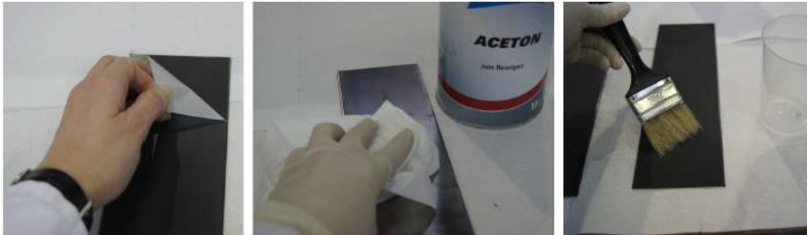
Figure 2.5: Surface's preparation and cleaning
