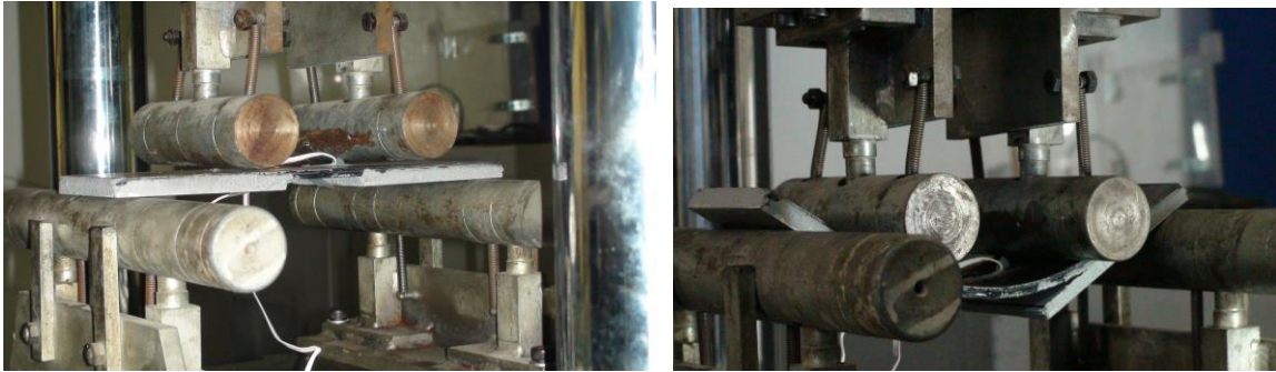
Figure 2.19: Specimen before and during testing (CFRP on the tension side)
