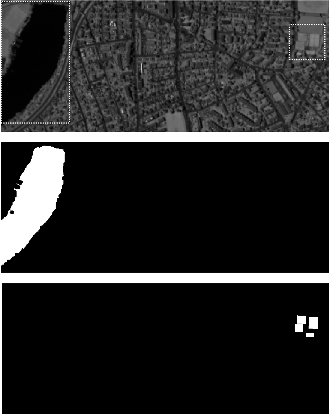
Figure 5.2 Regions of interest and ground truth map for a. Water b. Tennis courts
