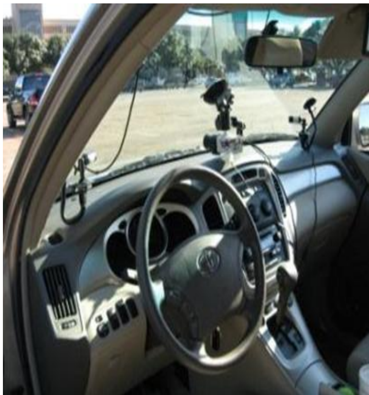
Figure 2.4. An instrumented vehicle used for on-road studies
