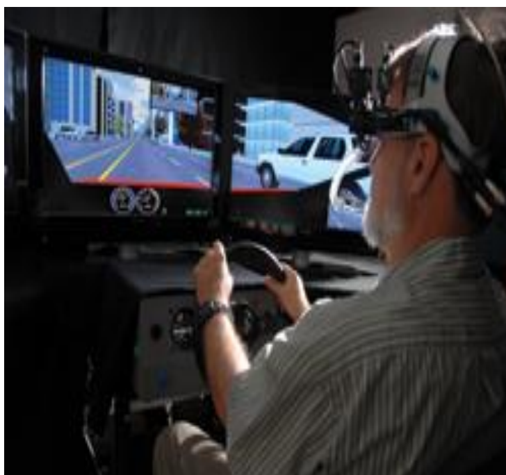
Figure 3.3. Head-mounted device tracks the eye movements
