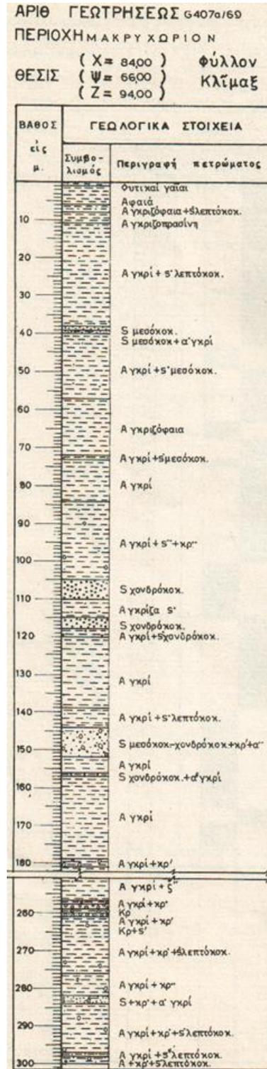
Figure 19: Geological logs of G403 and G407 monitoring wells in group 3 of Karditsa. Most clay is encountered.
