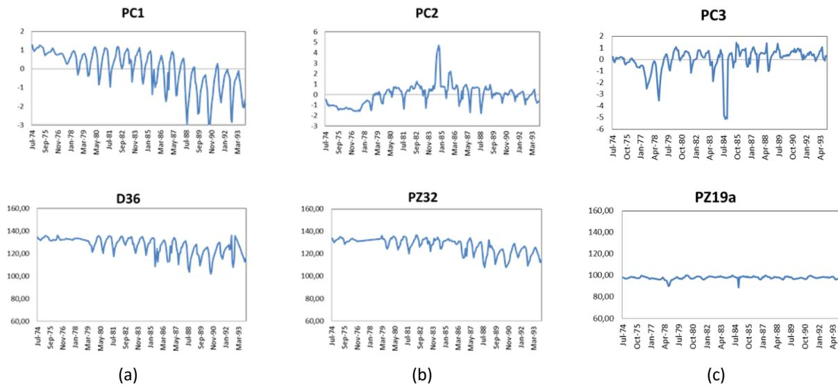
Figure 15: Component scores plot and hydrographs of representative monitoring wells for the three principal components in Karditsa.
