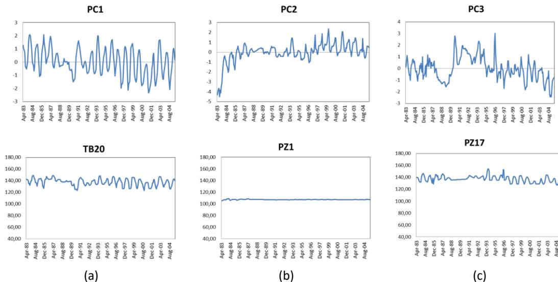
Figure 24: Component scores plot and hydrographs of representative monitoring wells for the three principal components in Trikala area.
