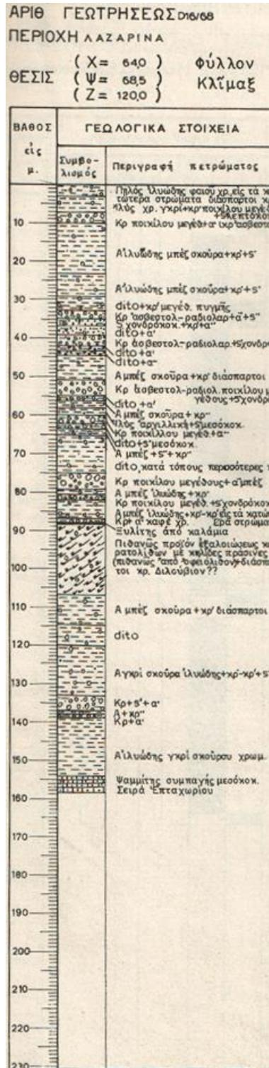
Figure 27: Geological log of monitoring well D16 in group 2 of Trikala. Mostly clay and sand are encountered.
