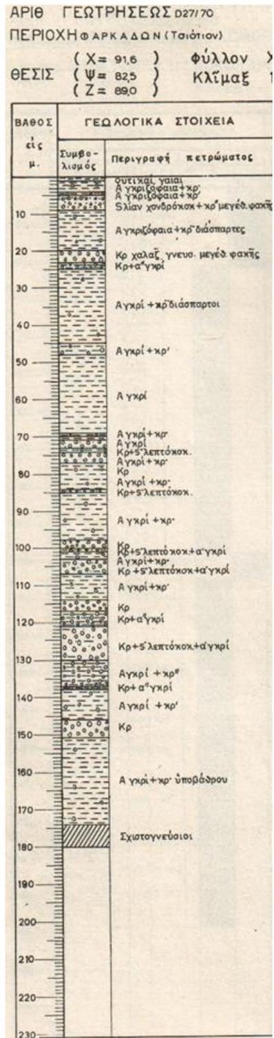
Figure 26: Geological logs of D25 and D27 monitoring wells in group 1 of Trikala. Mostly clay and gravels are encountered
