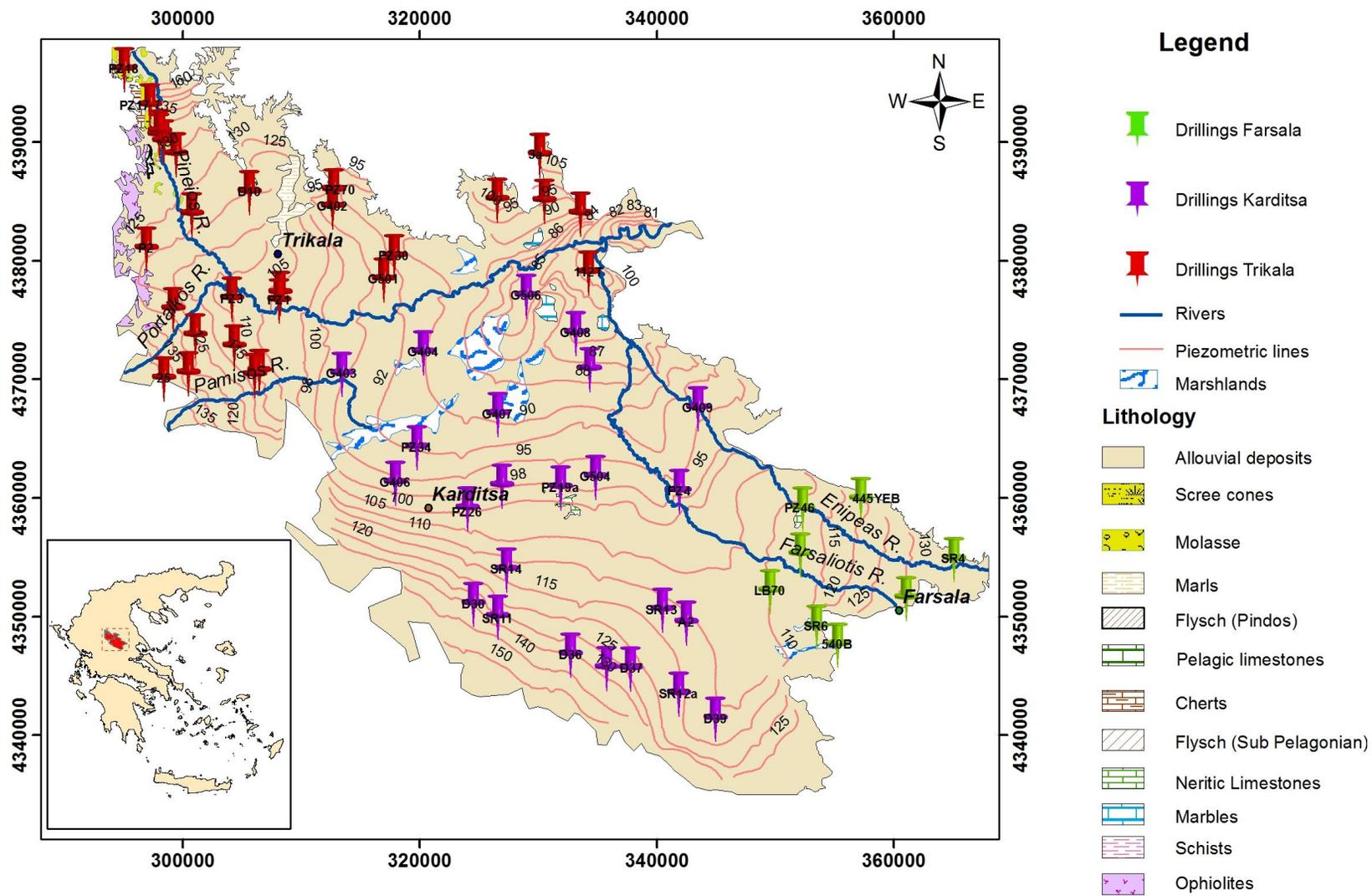
Figure 4: Geological and piezometric map of the West Thessaly basin.
