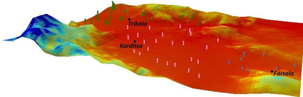
*Figure 6: DTM of West Thessaly basin showing the classification of data in three groups according to topography.*
