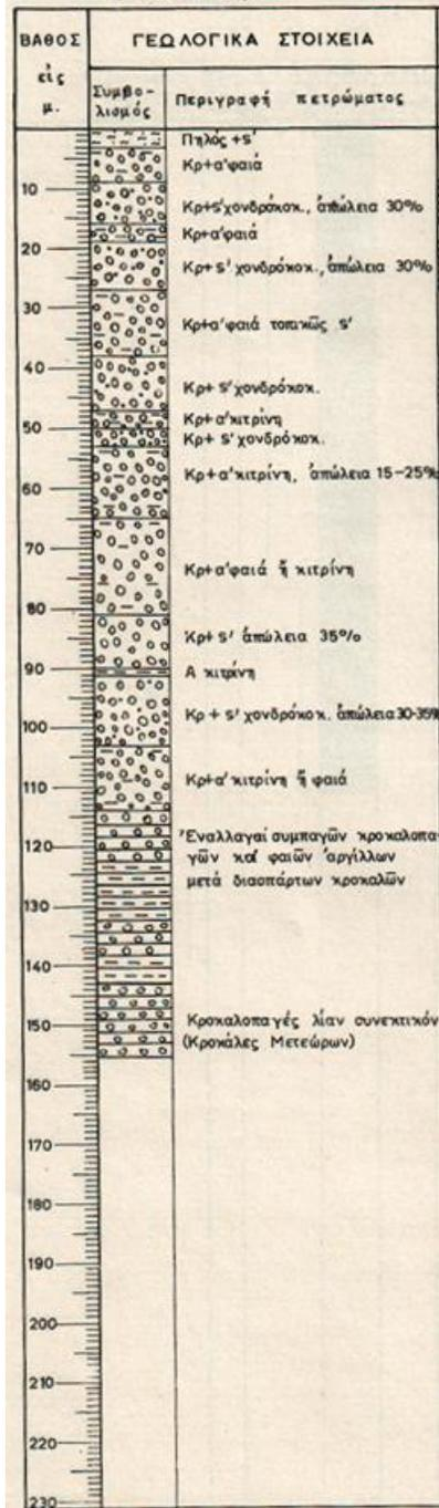
Figure 29: Geological log of monitoring well D2 in group 3 of Trikala. Mostly clay and gravels are encountered.
