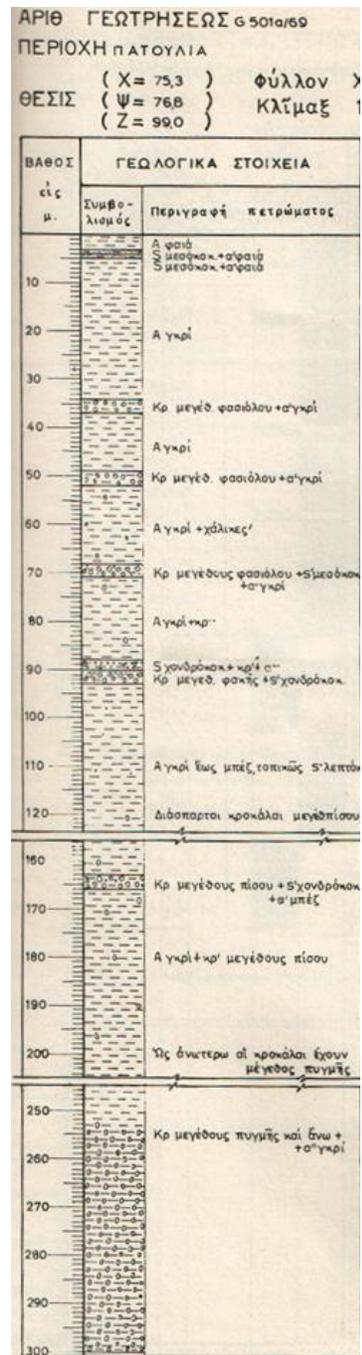
Figure 28: Geological logs of monitoring wells G402, G405 and G501 in group 2 of Trikala. Mostly clay and sand are encountered.
