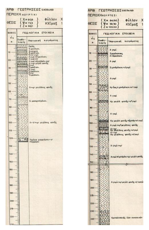
Figure 20: Geological logs of G408 and G503 monitoring wells in group 3 of Karditsa. Most clay is encountered.
