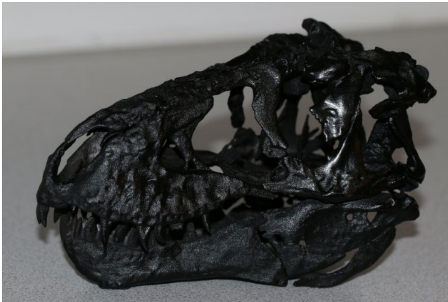
T. rex Head: 1:10 scale selective laser sintering print of photogrammetric model 52
