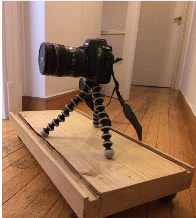
Movable Platform for the Camera Rig
