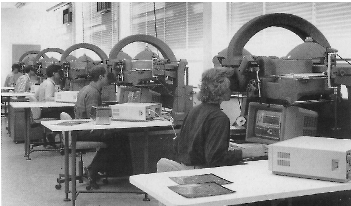
Analytical Conversion of Wild B8 stereo-plotters
