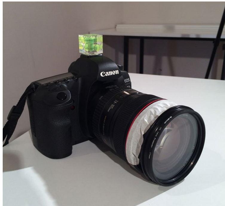
Camera with 3-axis leveller and zoom lens, taped at chosen focal length
