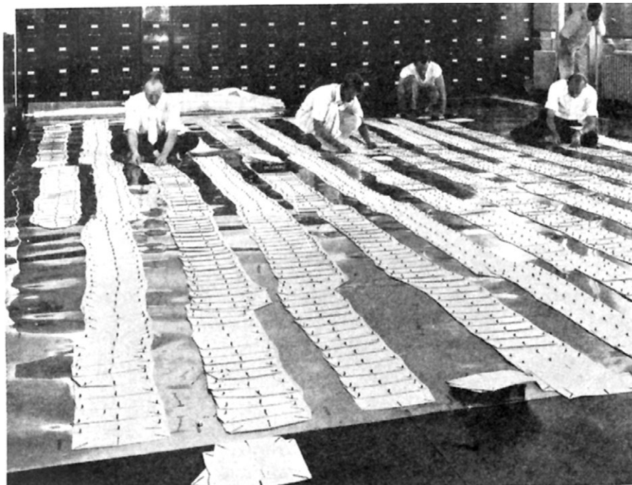
Slotted templates being laid at the Soil Conservation Service, U.S. Department of Agriculture. 8
