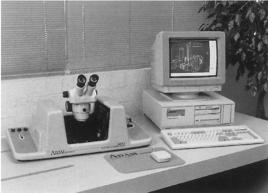
The ADAM MPS-2 analytical plotter
