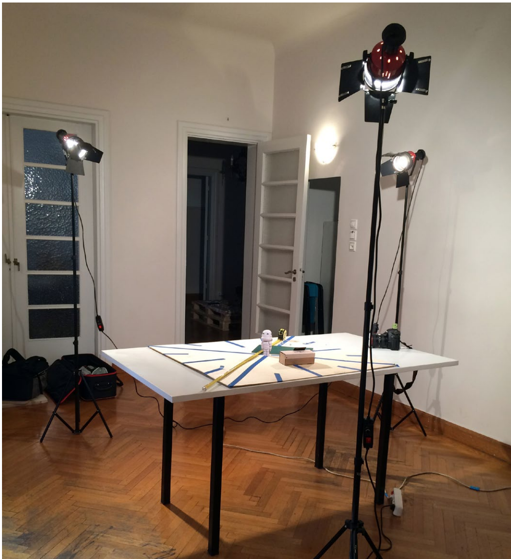
3 Lights set-up with dimmer control at triangle formation and intensity/direction for shadow control
