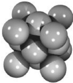
(α) Face centered cubic lattice
