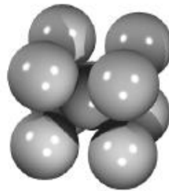
(β) Body centered cubic lattice
