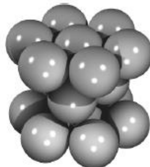
Hexagonal close packaged structure (lattice representation – sphere model)
