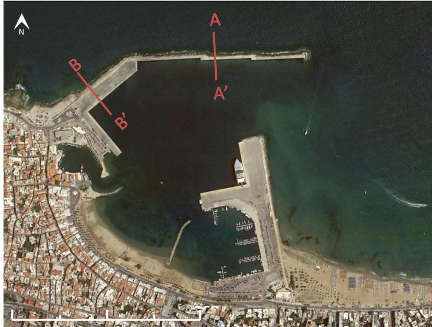
**Figure 10** The two known sections of the breakwater used for the estimation of wave overtopping.
